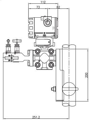
5-way manifold valve at bottom and multi-planer process connection
