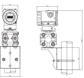
PAD standard with flat type bracket (vertical mounted)\*
