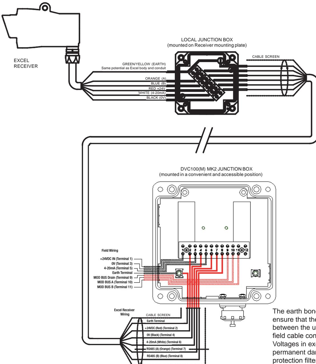
The earth bonding arrangement must ensure that the maximum peak voltage between the unit case earth and any field cable conductor is less than 350V. Voltages in excess of this can cause permanent damage to the unit's RFI protection filters.
