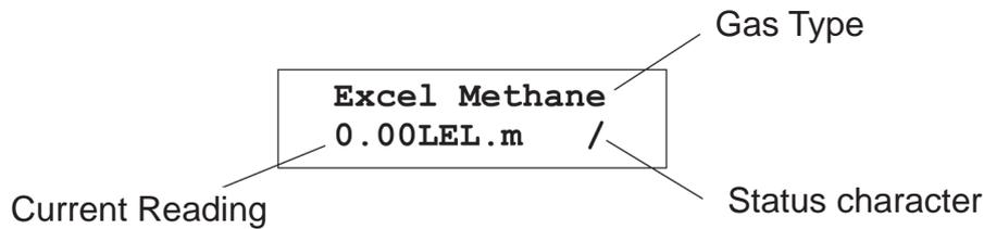
*The first line of the display shows the name of the gas or its identifier in a special gas table.*
