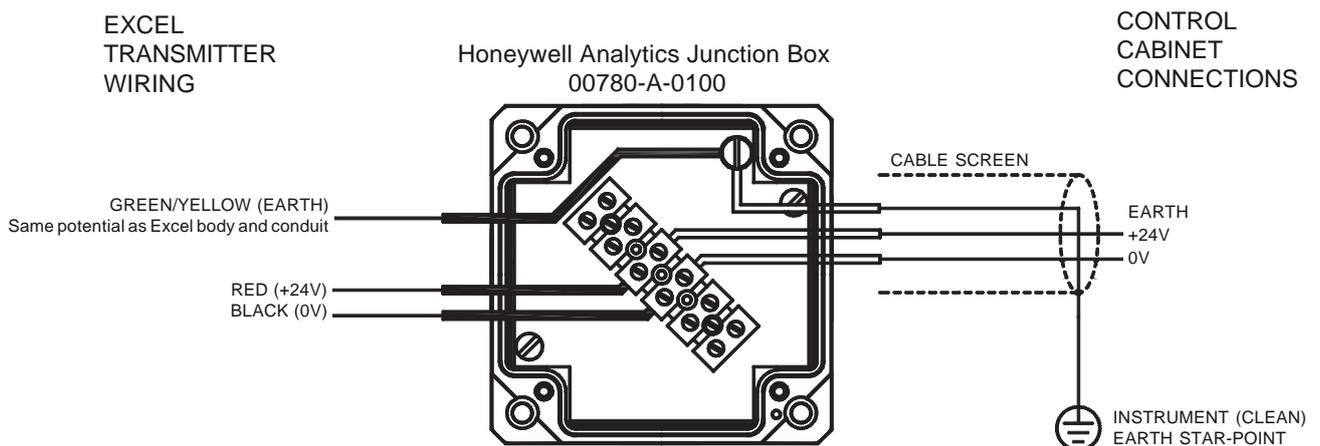
The earth bonding arrangement must ensure that the maximum peak voltage between the unit case earth and any field cable conductor is less than 350V. Voltages in excess of this can cause permanent damage to the unit's RFI protection filters.
