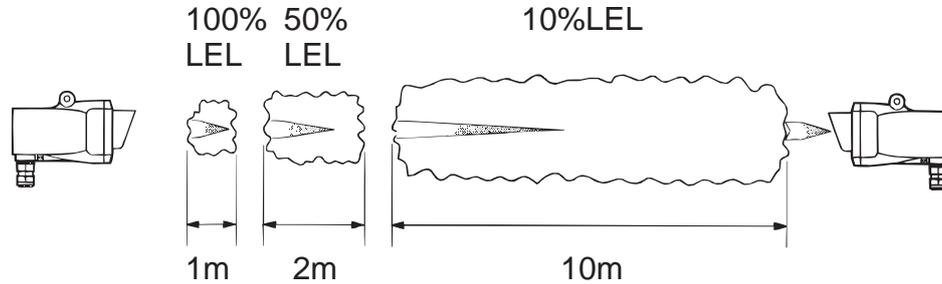
LEL.m monitoring is particularly beneficial while the Excel gas detector is protecting the perimeter of a plant or process, often reducing the quantity of point detectors required. The open path LEL.m system has the ability to detect leaks that point detectors may miss due to prevailing or changing wind directions, and can provide early warning of a dilute gas cloud when point detectors may not register any gas presence.
