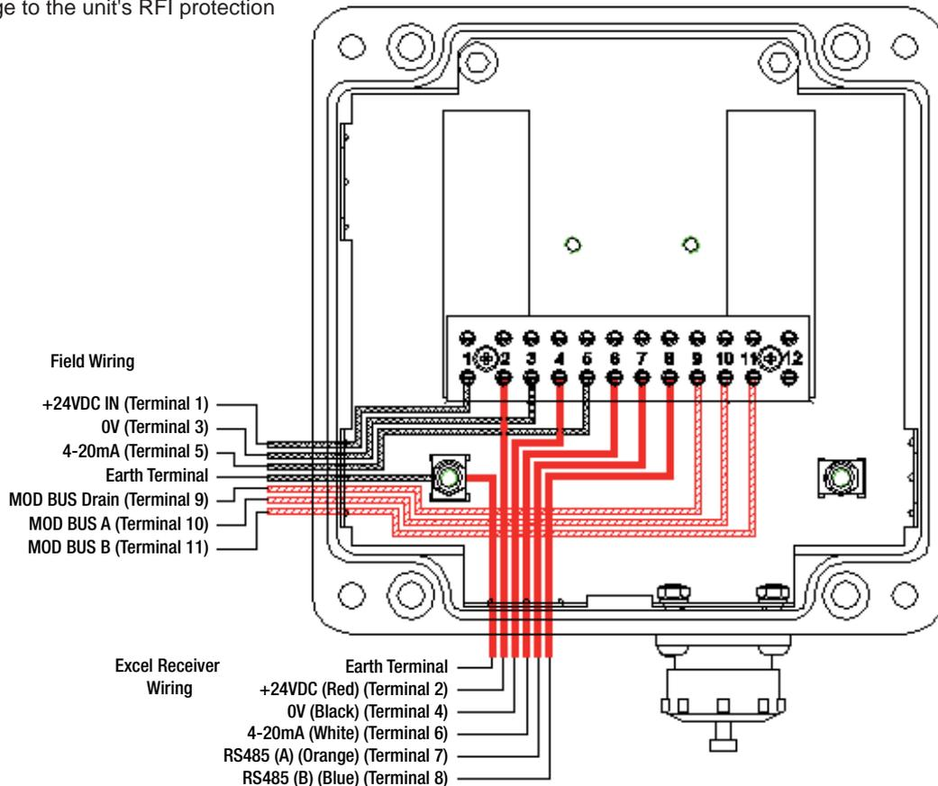
Note: Using metal cable glands will connect the screen of the cable to the Excel Body.
