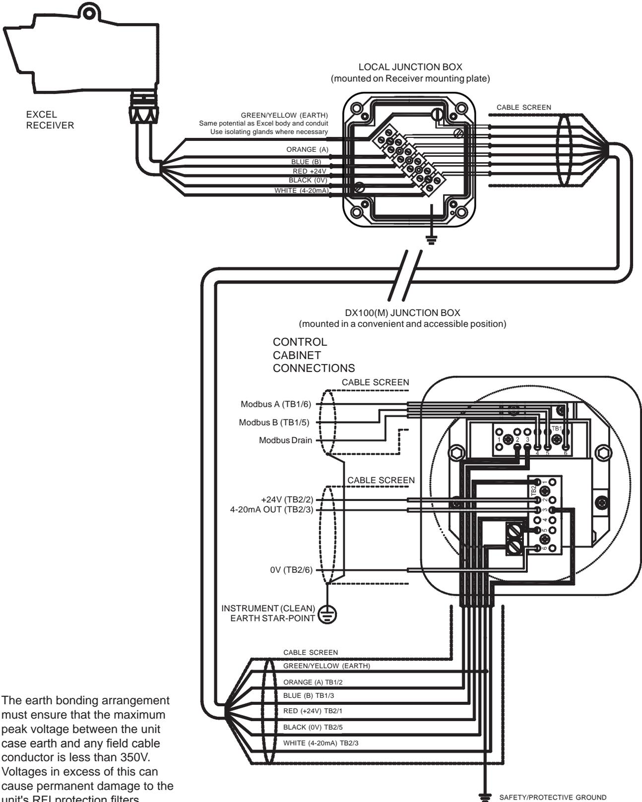
The earth bonding arrangement must ensure that the maximum peak voltage between the unit case earth and any field cable conductor is less than 350V. Voltages in excess of this can cause permanent damage to the unit's RFI protection filters.
