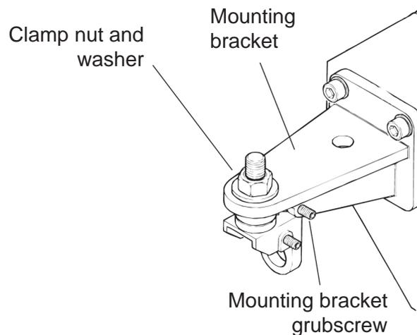
***Do not fully tighten the nut (Refer to 3.73).***
