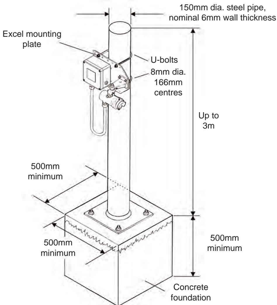
*Note: The pipe can be filled with concrete to provide extra robustness if necessary.*
