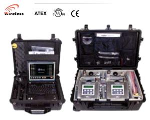
The Rapid Deployment Kit (RDK) is a complete solution designed for quick assessment of gaseous and radiation threats. The kit includes four wireless 5-gas AreaRAE detectors with in-case charging, and a Host Controller for monitoring from a command center up to 2 miles (3 km) away. The system can scale up with the addition of Detector Kits, each containing four AreaRAEs.
