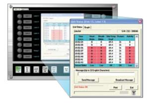
ProRAE Remote provides a simple yet powerful solution that integrates the outputs of remote AreaRAE-family sensors into user-friendly displays on a PC. It facilitates real-time wireless communication from up to 64 remote monitors to a host computer up to 2 miles (3 km) away. With the GPS option, the sensor data is displayed on a multi-layered mapping area with detailed and accurate representation of streets, highways, railroads, rivers, and borders.
