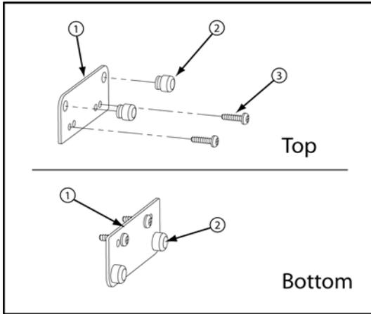
**Figure 18. Parts of the Wall Mounting Plate**
