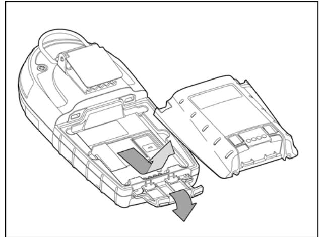
**Figure 9. Removing the Micro 5/PID/IR Lithium Battery Pack**
