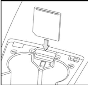
**Figure 25. Replacing a MMC/SD Card**
