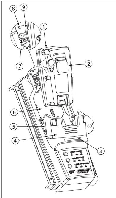
**Figure 11. Inserting the GasAlertMax XT**
