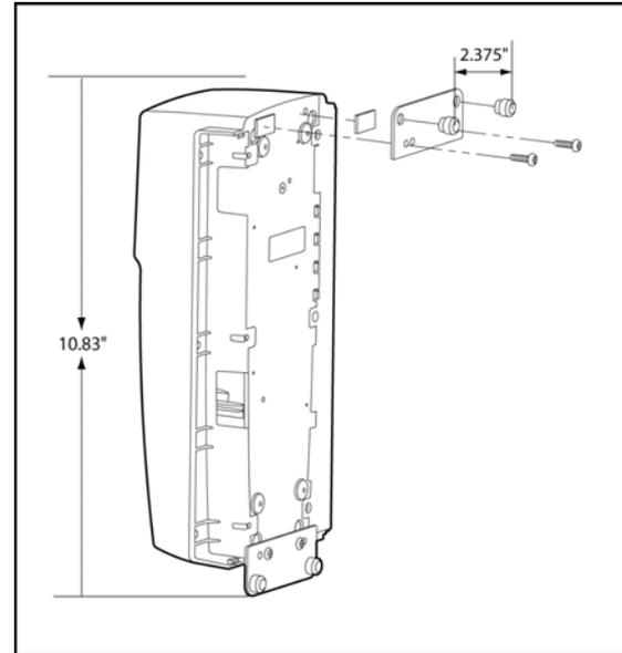
**Figure 17. Attaching the Wall Mounting Plate**
