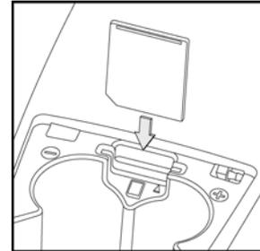
**Figure 21. Inserting the MMC/SD Card into the Base Station**
