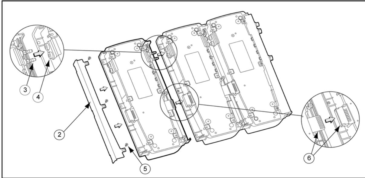
**Figure 15. Adding Another Docking Module (Back View)**
