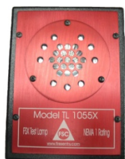
Figure 4-1 TL-1055 Hand Held Test Lamp (NEMA 1)
