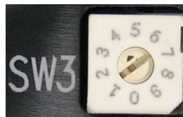
Figure 3-3 SW3 Ten (10) Position Rotary Switch
