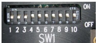
Figure 3-1 (SW1) Ten (10) Position DIP Switch
