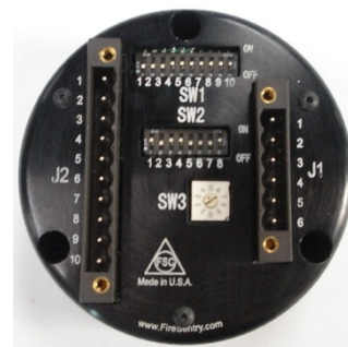
Figure 1-2 FS20X Detector Puck, (rear view)
