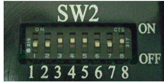
Eight (8) position DIP Switch (SW2) - Figure 3-2
