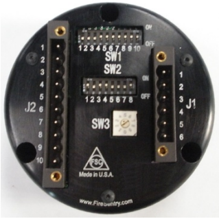
Figure 2-10 Detector Module “puck” (rear view)
