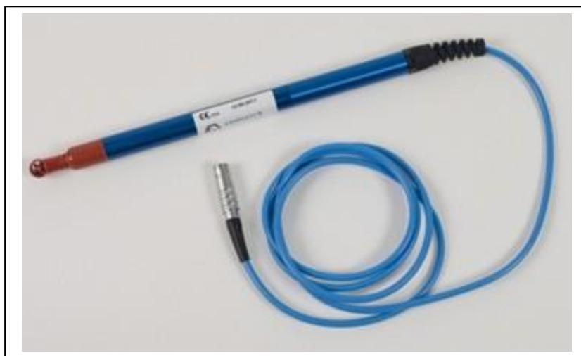
The GEM5000 gas analyser has the facility to attach an anemometer device enabling the site engineer to measure the flow of gas within an extraction system. The anemometer can be set to display two values; m/s (meters per second) and m<sup>3</sup>/hr (metres cubed per hour).
