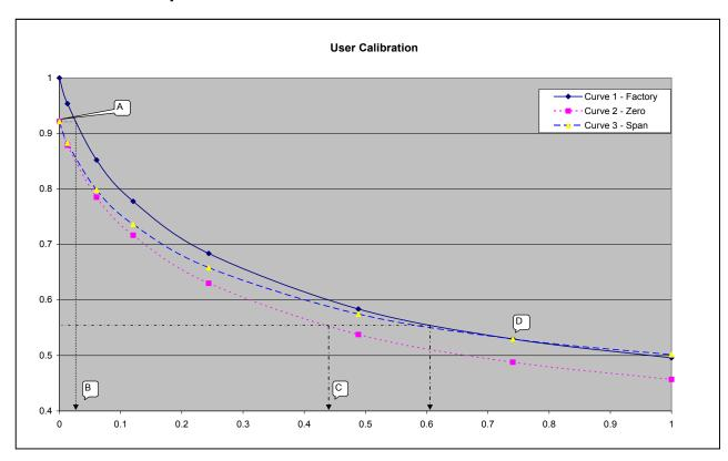
User calibration is a means of optimising the performance of the instrument to the current operating conditions such as ambient temperature and pressure as well as correcting for instrument drift caused by lamp and filter settling.
