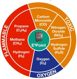
two gases simultaneously and cost effectively, in any of the following combinations: toxic-toxic, toxic-combustible, oxygen-toxic, or oxygen-combustible.
