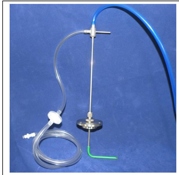
Example of a pitot tube
